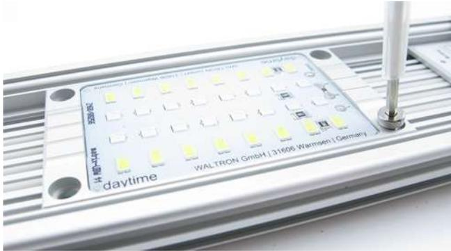
Loosen and remove all screws.
